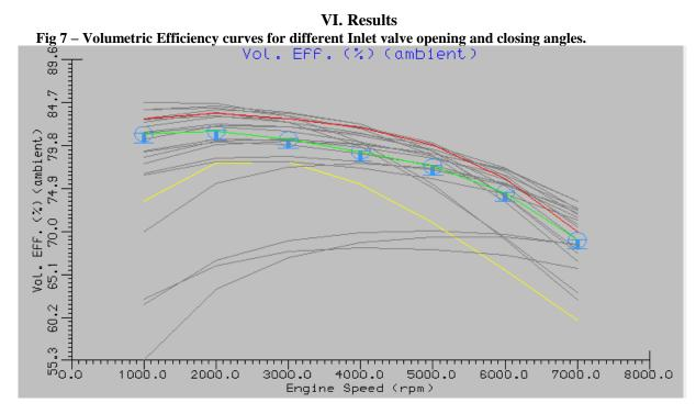
The optimum 9 curves in **Fig.2**earlier are selected from these curves. Variation of Valve timing done: IVO: 0-50<sup>o</sup> IVC: 0-90<sup>o</sup>Valve Lift: 6-12mm Red Line- Overall best Values Green line- Default Engine Values Yellow line- Picked Value (Current)
