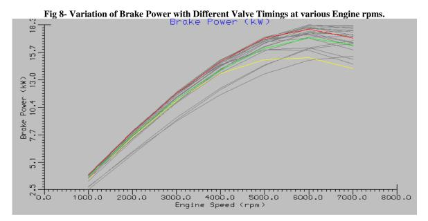
The above Graph indicates that Brake Power, BSFC and BMEP are indeed dependent on the Volumetric Efficiency as the graph with higher BP indeed is the one with higher Volumetric Efficiency (Red)
